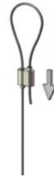
3. Insert cable back into looping cable lock. Cable must exit looping cable lock minimum 1 inch.
